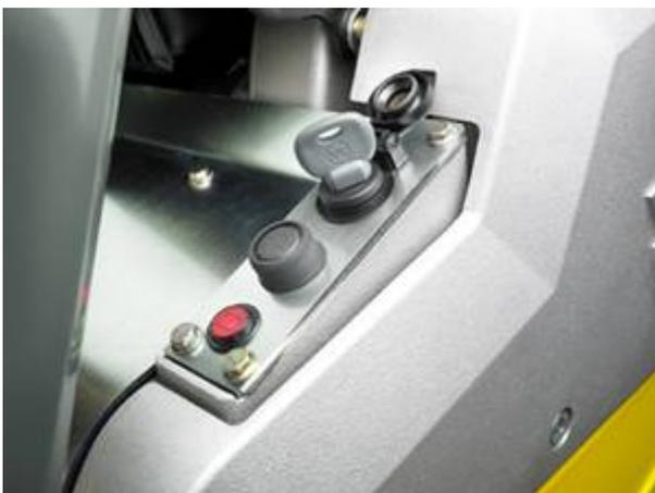
Simply use an ignition key to start the model with electric starter.
