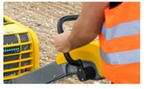
• Operator safety: If the operator releases the center pole the vibratory plate continuous vibrating but remains in place (on-the-spot vibration)
