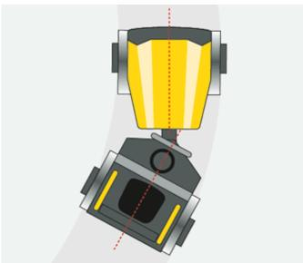
**Uniform compaction, optimal driving stability:** The three-point articulated pendulum joint ensures a uniform weight distribution on the front and rear drum at all times. This also improves the maneuverability and provides for maximum stability when turning curves.
