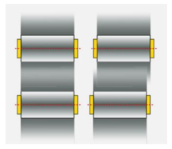
**The drum offset** allows for easy maneuvering when compacting along walls. In crab steering, the roller can be conveniently controlled in any desired direction.
