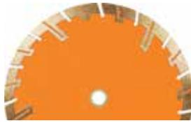
Premium quality Turbo rim blade for cutting softer type materials giving fast efficient cutting with extended life. Types of materials recommended for cutting include concrete blocks/pavers, sandstone and aerated concrete. Can be used both wet or dry.
