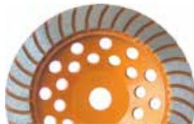
Turbo diamond cup wheel with a coarse grit diamond designed for rapid removal of a wide range of construction materials with exceptional life. Materials include concrete, bricks, concrete pavers, stone, concrete blocks etc. Should be used dry on electric power tools.
