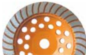
Turbo diamond cup wheel with a medium grit diamond designed for removal of a wide range of construction materials without deep scratching and giving exceptional life. Materials include concrete, bricks, concrete pavers, stone, concrete blocks etc. Should be used dry on electric power tools.
