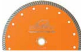
Thin turbo blade for fast chip free cutting of very hard materials including ceramic and porcelain tiles, clay bricks, marble and slate. Commonly used on angle grinders in dry application.
