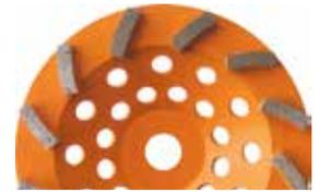
Spiral diamond cup wheels available with 9, 12 and 24 segments for aggressive grinding to more controlled type application where extended life is desired. Should be used dry on power tools or wet/dry if used on a walk behind floor grinder. Suitable for grinding concrete, bricks, concrete pavers, stone, concrete blocks etc.
