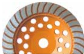
Turbo diamond cup wheel with a fine grit diamond designed for fine grinding or removing scratches and finishing off on a wide range of construction materials and giving exceptional life. Materials include concrete, bricks, concrete pavers, stone, concrete blocks etc. Should be used dry on electric power tools.
