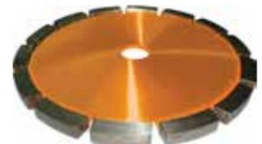
Premium quality 9.5mm wide blade used for tuck pointing and cleaning of mortar joints. Most commonly used by the professional in dry application.
