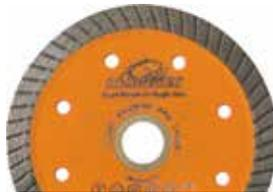
Turbo rim blade used in a variety a general purpose cutting applications where a chip free cut is not required. Used for cutting materials such as clay and concrete bricks, cement sheet, general concrete (not reinforced), concrete roof tile and clay/concrete pipes. Can be used both wet or dry.
