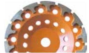
New design "R" segment designed for rapid removal of concrete and hard painted coatings which have been applied to concrete Should be used dry on power tools or wet/dry if used on a walk behind floor grinder.
