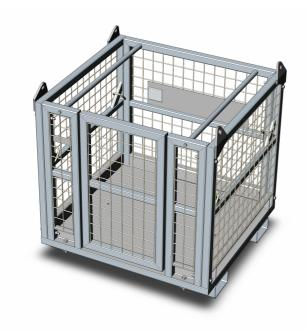
The type WP-NC Crane Cage Work Platform has been designed strictly in accordance with Australian Standard AS 1418.17 and is suitable for a maximum of four people. Work performed in this Cage shall be limited to special tasks of short duration in situations where necessary to elevate personnel where it is not practicable to erect scaffolds or use a specially designed device. Fork Arm slippers are provided for transport purposes only. The standard finish on the Cage is Zinc finish.
