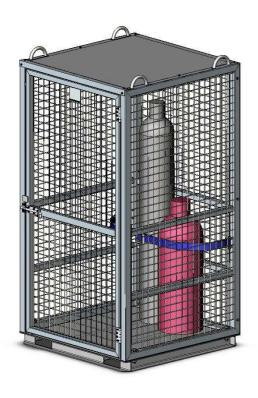
The type GB-CM2 Gas Cylinder Storage Cage has been designed primarily as a secure storage unit for building sites and mines. The lockable gate, mesh sides and roof sheeting ensure cylinder and gear security. The Cage is fitted with a 4 point Crane lift and Forklift pockets underneath for transport. The internal loadbinder prevents cylinder movement during transport.
