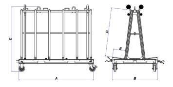
The CRL One Stop A-Frame is designed for transporting material and storing it in the factory or on the job site. The glass sheets are placed on special rubber profiles and secured with four (4) ratchet securing bars. The center section can be used to store tools and equipment.
