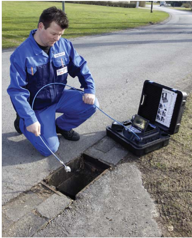
The 30m push rod and the pan&tilt or 26mm straight view camera head color camera head make sure nothing in the house supply line remains hidden from your view.
