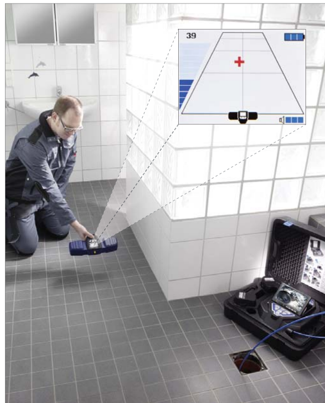
The actual meter count and the position of the head are displayed in the monitor. The Wöhler L200 8.9Khz Locator makes it possible to locate the camera head wirelessly.
