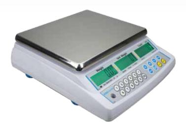
The CBC bench counting scale offers intelligent functions that are practical for any counting application. The intuitive software is user-friendly and keeps track of the count, automatically optimising the unit weight for greater accuracy. Designed to be tough, the CBC features ABS housing, stainless steel platform, non-slip feet and load cell protection. RS-232 interface allows easy communication with computers and printers.
