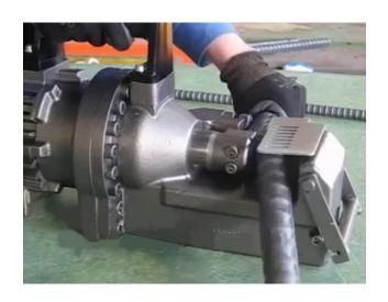
Big and tough, portable cutter which cuts any rebar up to and including 32mm.
