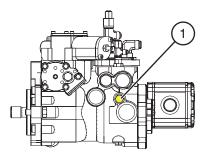
Figure 2-13. Drive Bypass Valve
