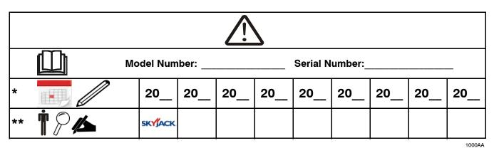
As described earlier in this section, this decal is located on the scissor assembly. It must be completed after an annual inspection has been completed. Do not use the aerial platform if an inspection has not been recorded in the last 13 months.
