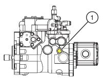
Figure 2-2. Drive Bypass Valve
