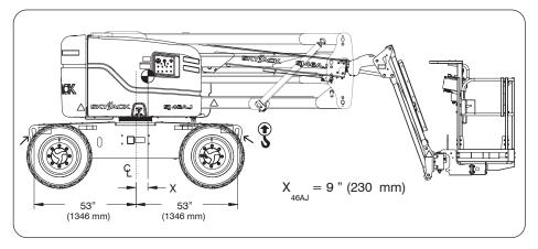
Figure 2-12. Lifting Points NOTE: Center of gravity varies with different options.
