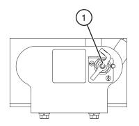
Figure 2-1. Main Power Disconnect Switch
