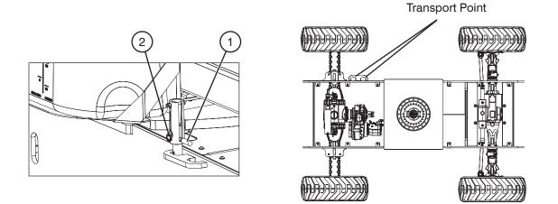
Figure 2-11. Turret Transportation Lock & Locking Points
