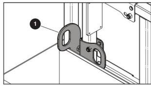
Fall-protection anchorage: When required, use this as a point to attach personal fall protection equipment (PFPE). Do not attach the PFPE to any other points on the platform. Do not use this anchorage to lift, anchor, attach, or hold the platform, or other apparatuses or material.
