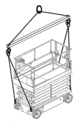
Figure 16 Appropriate method to hoist
