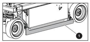
1 Pothole protection: This device consists of a set of mechanically actuated steel weldments located under the base. These weldments will automatically deploy for reduced ground clearance when elevating the MEWP. If the pothole-protection device has not fully deployed when the MEWP is in the elevated travel position the drive function will be disabled.
