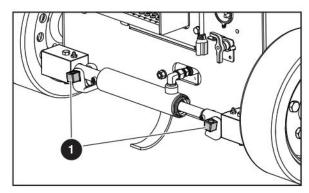
Figure 02 Brake release block (pin brakes)
