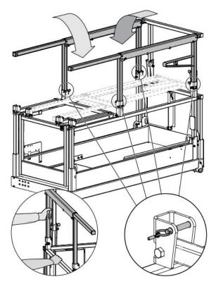
Figure 23 Left and right guardrail folded
