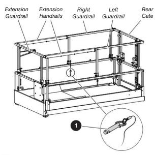
**1** Guardrail lock-pin with lanyard: Use this pin to lock the guardrails. Refer to Section 6.9.
