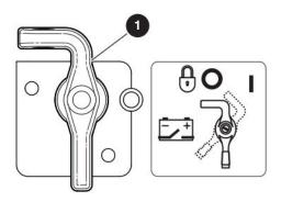
Main power disconnect: This switch disconnects power to all control circuits when in the off position. The switch must be in the on position to operate the MEWP. The switch must be in the off position when you transport the MEWP or put it in storage.
