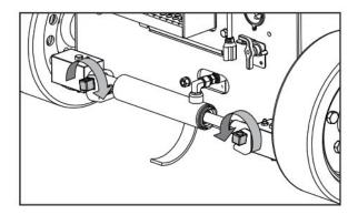
Figure 13 Brake release block (pin brakes)
