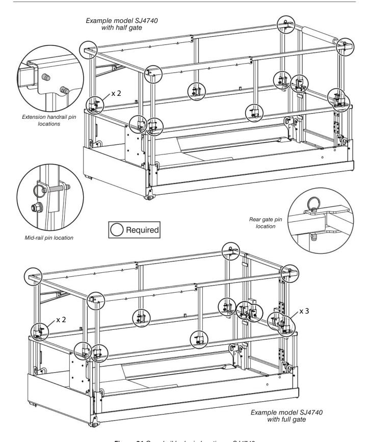
Figure 21 Guardrail lock-pin locations - SJ4740
