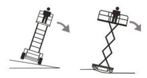
Do not depend on the tilt alarm as a level indicator.
