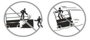
Machine must be on level surface or secured before releasing brakes.
