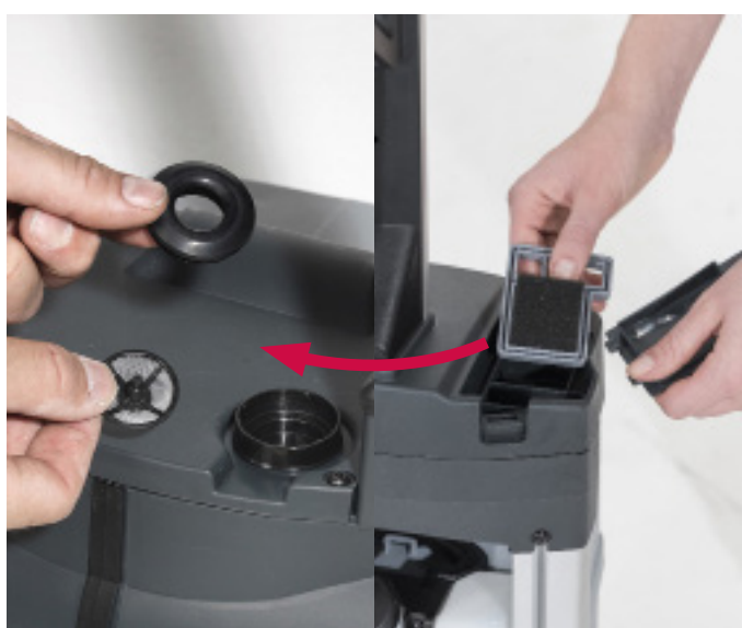
16. Check and clean the solution and vacuum filter regularly.
