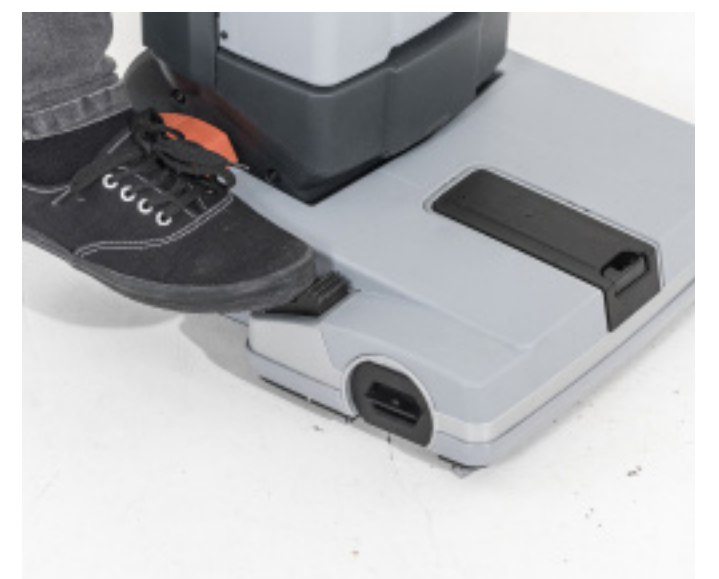
10. For double scrubbing, use the pedal to lift/lower squeegees.
