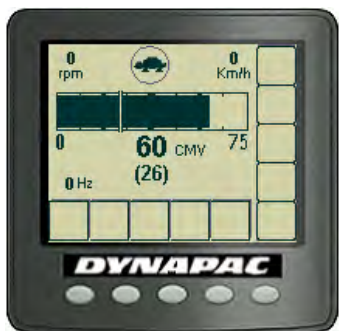
Fig. Compaction meter display (CMV display)
