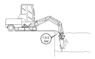
NOTICE When operating under water the hydraulic breaker must be fed with compressed air to keep the area between the piston and the inserted tool free from water. If the area between the piston and the inserted tool gets filled with water, it may penetrate into the hydraulic oil system when the hydraulic breaker is started.
