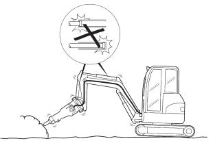
Avoid idling strokes; it causes wear on both working tool and tool retainers.
