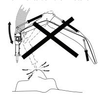
Never use the hydraulic breaker to move debris.
