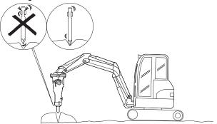
The hydraulic breaker or the working tool is not to be used as a lifting device. When lifting heavy components use the hook on the carrier arm.
