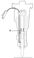
Lubricate the insertion tool's shank plentifully during all upward operations. The bushing and the insertion tool must be lubricated so frequently that dirt cannot penetrate into the hydraulic breaker. When the insertion tool is exposed to high pressure and high temperatures a standard type of grease will melt and run. To avoid this always use Atlas Copco chisel paste.
