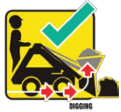
Towards the end of the run when the bucket is nearly full, gently tilt the bucket (rotate the bucket) towards the Loader. This decreases the lifting resistance when the arms are raised and promotes an efficient tear out.
