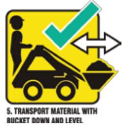
The material may then be dumped into a trailer or utility truck for removal or repositioning on the site.
