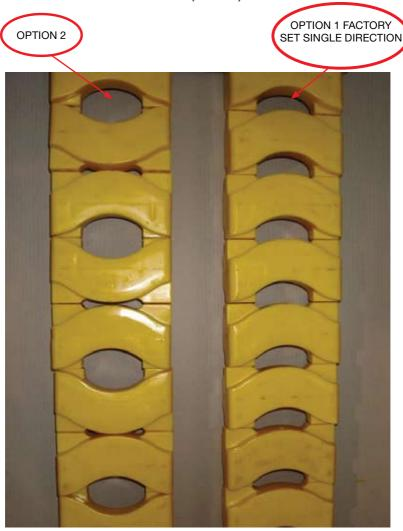
Follow these instructions to change the option, start by removing the tracks from the machine; use the **Track Removal Instructions** to perform this operation.
