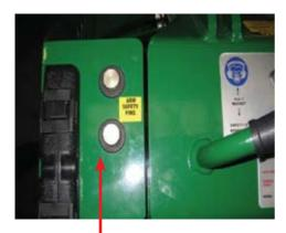
LOCKING PINS ARE KEPT TO THE LEFT SIDE OF THE CONTROLS.
