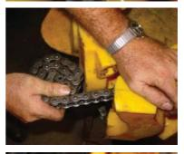
4. Lay segments out on the floor in the required pattern, and then feed the chain in from one end through to the other. It will assist if the chain is washed clean and soaked in diesel. If you have trouble, you can thread a piece of 3 mm wire in from the other end and connect it to the chain to help pull the chain through.
