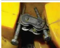
3. Pull the locking bolts out and remove the chain simply by pulling it through the track segments. Then turn the track onto it's other side and repeat steps 1, 2 and 3.
