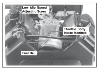
Figure 22. EFI Throttle Body Manifold.
