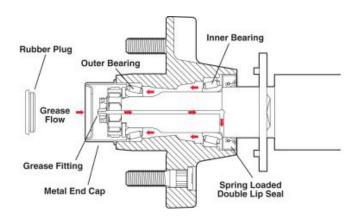
Axles equipped with Dexter's E-Z Lube feature can be periodically lubricated without removing the hubs from the axle. This feature consists of axle spindles that have been specially drilled and assembled with grease fittings in their ends. When grease is pumped into the fitting, it is channeled to the inner bearing and then flows back to the outer bearing and eventually back out the grease cap hole.
