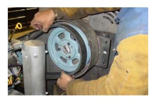
ALWAYS REMEMBER TO REPLACE BELT GUARD COVER BEFORE STARTING MACHINE. ROTATING BELTS AND SHEAVES ARE DANGEROUS AND COULD SEVERELY INJURE SOMEONE.
