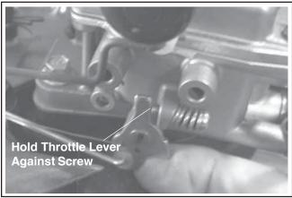
Figure 19. Holding Throttle Lever Against Idle Stop Screw.
