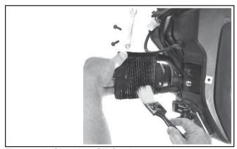
Figure 10. Cleaning Oil Cooler.
