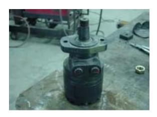
• Attach the torque arm to the new motor using the 1/2" bolts that were removed. Tighten the bolts and torque to 120 ft. lbs. (The torque arm looks slightly different on the lower feed motor, but is still held on with two bolts.)
