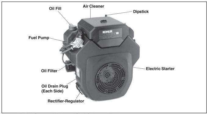
Figure 1. Typical Command Horizontal Shaft Carbureted Engine.
