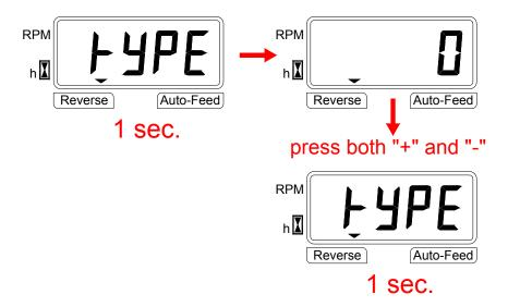
The parameter is changed by using key "+" or "-"; switching key "PROG" allows to go to next parameter "BACK" (i.e. activation time of the reverse solenoid valve, in ms). It is displayed with same procedure.
