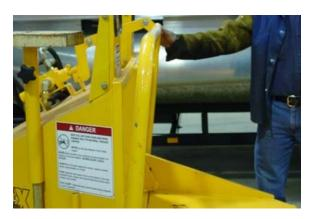
Push the throttle over into the low position so that the engine can slow down then turn the key to the off position.
