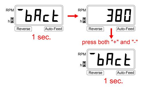
The parameter is changed by using key "+" or "-"; switching key "PROG" allows to store all data entered and quit setting - the display will show for 1 second following indication:
