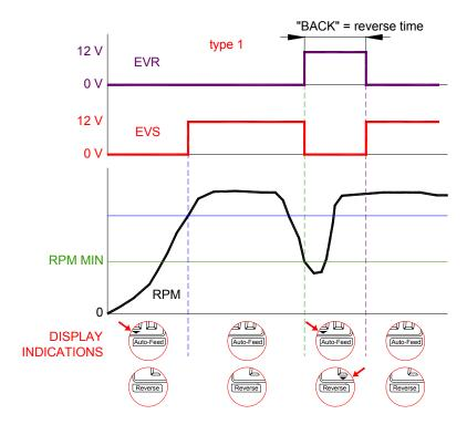
During operation, working hours can always be displayed by switching for a BRIEF INTERVAL key (+) or (-). The display shows now the ref. indicator "b" on page 7 and working hours are displayed for 3 seconds. During this interval the EVS solenoid valve is energized or de-energized by the monitor (according to what programmed in "type" parameter) only if the "auto-feed" function has been enabled (see chapter 5.3), whereas the EVR solenoid valve is never energized.
