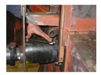
Reconnect the hydraulic hoses making sure to connect them in the right order, see markings made when hoses were removed. If hoses are reversed, the feed wheels will work in reverse. Change hoses if this happens to make feed wheels turn correctly.
