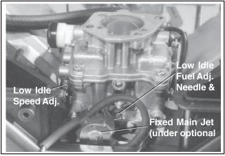
Figure 17. Carburetor (CH18-25, CH730, 740).
