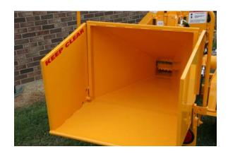
Locking the tray will prevent the tray being jerked closed by the brush being chipped and causing damage and possible injury.
