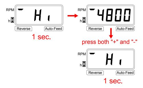
The parameter is changed by using key "+" or "-"; switching key "PROG" allows to go to next parameter "LO" (i.e. RPMs minimum permitted value). It is displayed with same procedure.
