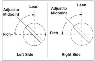
Figure 21. Optimum Low Idle Fuel Settings.
