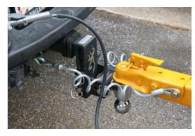
CHIPPER SHOULD RIDE AS CLOSE TO LEVEL AS POSSIBLE WHEN TOWING
