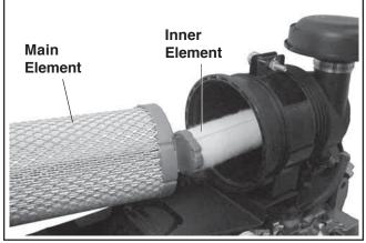
Figure 12. Removing Elements.
