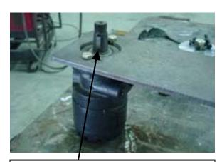
LINE UP KEY WITH KEYWAY ON COUPLING
