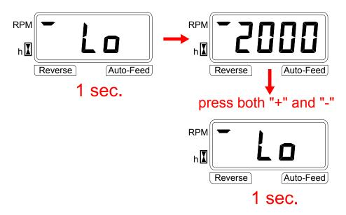
The parameter is changed by using key "+" or "-"; switching key "PROG" allows to go to next parameter "TYPE" (i.e. machine with reverse solenoid valve or without reverse valve). It is displayed with same procedure.
