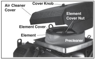
Figure 11. Air Cleaner System Components.
