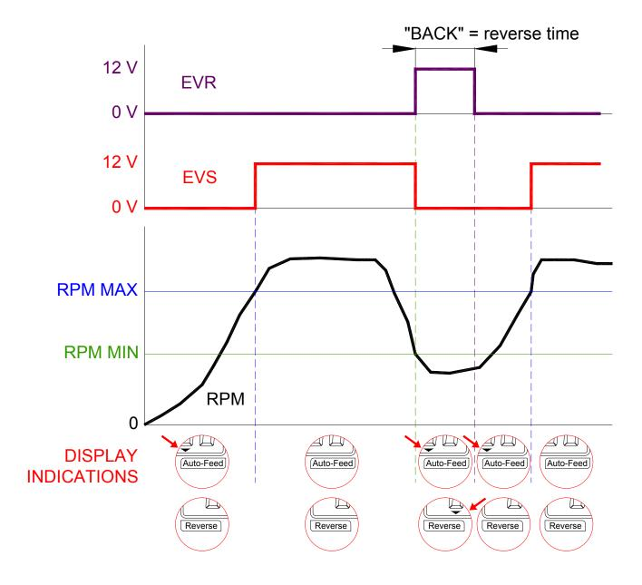
In case RPMs exceed the RPM maximum value during the reverse interval (back), the activation sequence shall be as shown below:
