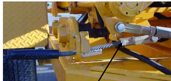
LOOSEN THE JAM NUT AND ADJUST THE SLIDE LOCK HANDLE
