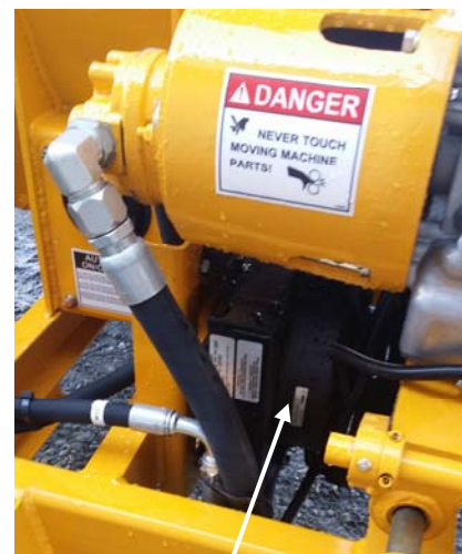
THE OIL COOLER IS LOCATED BEHIND MOTOR
