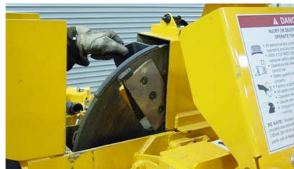
ROTATE CUTTER DISK TO CHECK FOR BINDING
