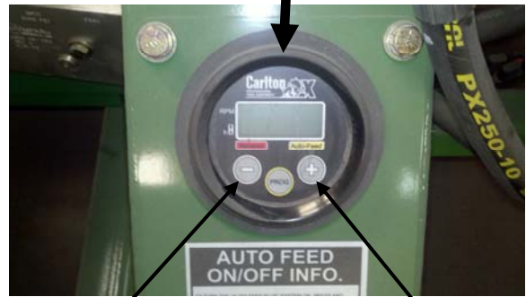
AUTO-FEED OFF (PRESS AND HOLD FOR 2 SECONDS TO TURN OFF)
