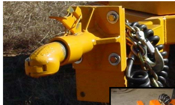
HITCH AVAILABLE IN 2" OR 2 5/16" COUPLER OR 2 1/2" PINTLE RING, PICTURED AT RIGHT.
