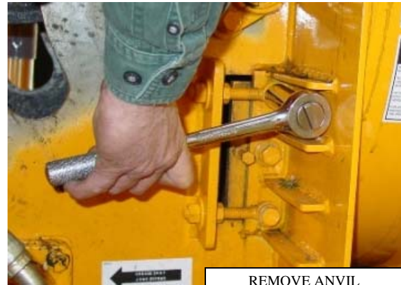
REMOVE ANVIL BOLTS & WASHERS
