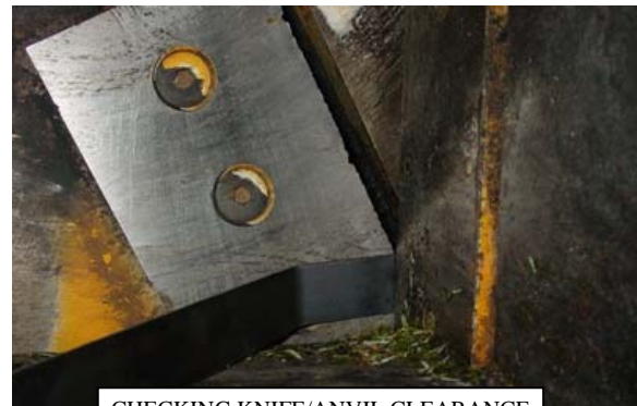
CHECKING KNIFE/ANVIL CLEARANCE
