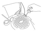
The oil filler cap must be completely screwed down to give a correct indication of the oil level.
