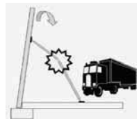
Construction overload from traffic, backfill, or another structure
