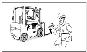
Remove the starter key and attach a sign saying DO NOT OPERATE.
