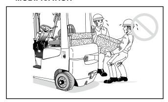
Modifications or additions that affect the capacity, construction or strength of the truck must not be performed by the user without the manufacturer's or his authorized representative's prior permission. For example, don't add a counterweight.
