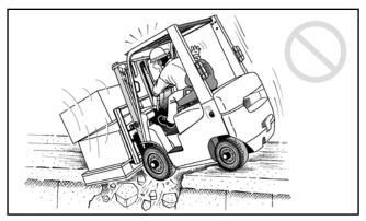
There is a fear of the edge of a soft ground breaking. Stay away from such a place. Keep appropriate distance from the edge of a narrow road or a platform.
