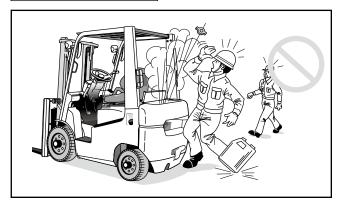
Immediately after the engine is shut down, the cooling water is hot and in high pressure.
