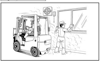
When the engine is run indoors such as in an enclosed warehouse, have a fresh-air ventilation. Exhaust fumes can cause chemical poisoning, and in the worst case exhaust fumes can kill. When warming up or operating the truck indoors, open the windows and doors or use a fan to make sure there is a good ventilation.
