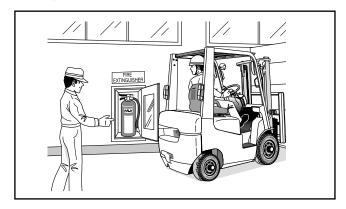
Fire extinguishers and first aid kits should be provided and maintained for use in case of a fire or accident. All personnel should understand the location and use of emergency equipment.
