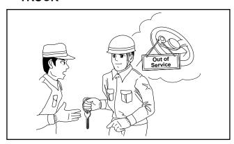
A truck that has not passed an inspection must never be operated. Hang a sign on the truck and remove the ignition switch, to make sure no one uses it. Then report the problem to the supervisor and wait for the repair to be completed.
