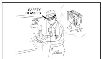
The battery electrolyte contains dilute sulfuric acid, a very corrosive material. It can destroy most things it touches. It will cause painful and serious burns if it gets on the skin. It can cause blindness if it gets into eyes. If battery electrolyte comes in contact with the skin or clothing, wash it away immediately with a copious amount of water.
