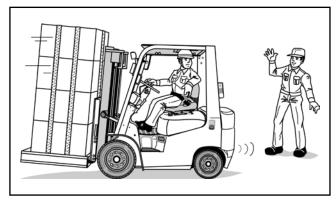
When handling bulky loads which restrict your vision, operate the truck in reverse and have a guide.
