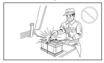
Do not short the battery terminals by placing a piece of metal between the positive and negative terminals. A loose terminal might cause sparks, causing an explosion. Make sure the terminals are tight. Use caution not to have the wrong connections of the battery terminals.
