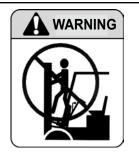
It is dangerous to use the truck body or mast as a ladder to ride on a high place.
