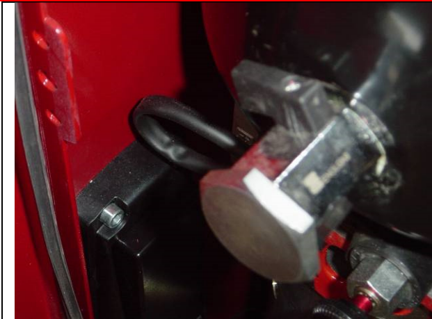
Illustration 4.0: Draining valve for the hydraulic oil.
