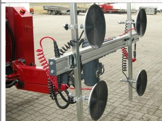
Illustration 6 All four suction cups must be regularly inspected for wear and tear. Never operate the machine with damaged suction cups.
