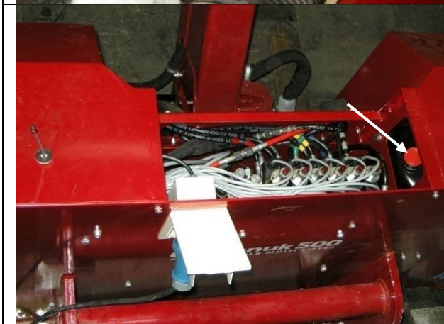
Illustration 3.0: Hydraulic station fill screw.
