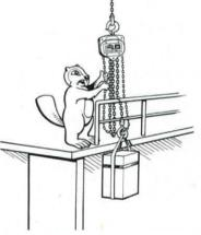
DO NOT operate the chain block unless it is rigged to pull in a straight line from hook to hook, and the frame is allowed to freely swivel on the upper hook.
