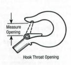
Any hook that is twisted or has excessive throat opening, indicates abuse or over loading of the unit. Other load sustaining components of the chain block should be inspected for damage. The chart above should be used to determine when the hook must be replaced. To measure throat opening, depress the latch against the hook body as shown above.
