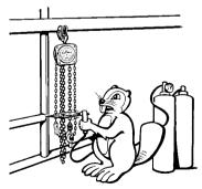
**DO NOT** heat treat and **DO NOT** weld any part of the chain block, expecially the load chain.
