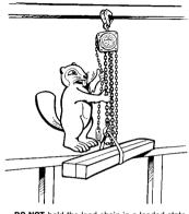
**DO NOT** hold the load chain in a loaded state while operating the chain block as serious injury may occur if the brake did not operate properly.
