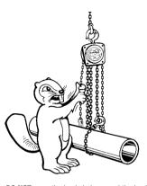
**DO NOT** wrap the load chain around the load and hook onto itself as a choker chain or bring the load in contact with the chain block.
