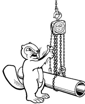
**DO NOT** wrap the load chain around the load and hook onto itself as a choker chain or bring the load in contact with the chain block.
