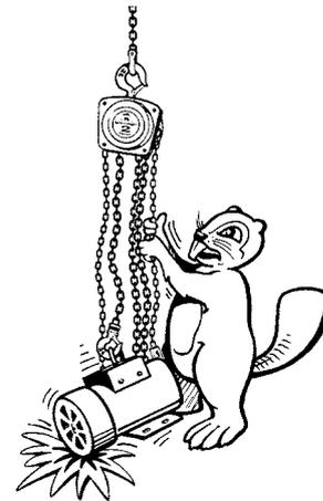
**DO NOT** shock load chain block, chain or hook.
