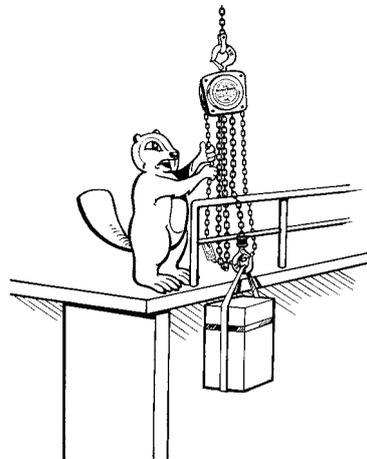
**DO NOT** operate the chain block unless it is rigged to pull in a straight line from hook to hook, and the frame is allowed to freely swivel on the upper hook.
