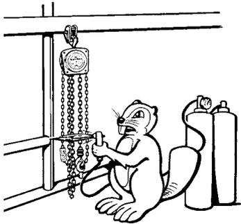
**DO NOT** heat treat and **DO NOT** weld any part of the chain block, especially the load chain.
