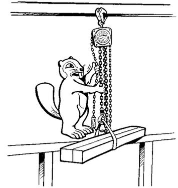
**DO NOT** hold the load chain in a loaded state while operating the chain block as serious injury may occur if the brake did not operate properly.
