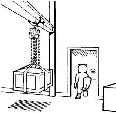
**DO NOT** leave a load suspended on the chain block unattended.
