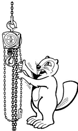
**DO NOT** run the hook assembly into the frame of the block.
