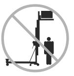
Do not stand under the load. The safety brake system (if equipped) will allow the load to drop 1 to 3 feet / 30 to 92 cm before locking the columns.
