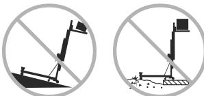
Prior to use, check the work area for drop-offs, holes, bumps, debris, unstable or slippery surfaces or other possible hazardous conditions. Do not raise the load unless the load handling attachment is properly secured to the machine.
