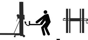
3 Adjust the forks to the desired width and be sure the snap pin is properly inserted in each fork.
