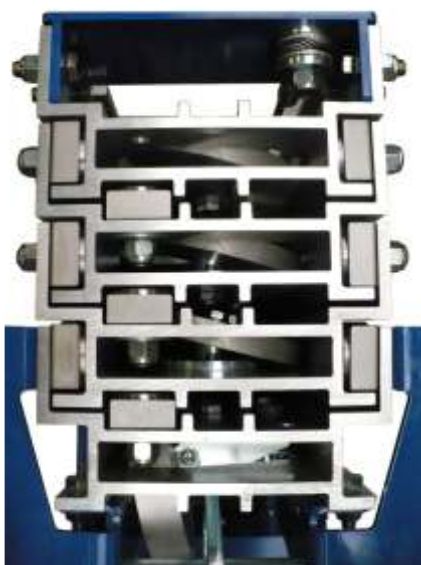
Mast system with special profiles and bearings
