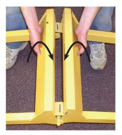
**4.** Lower the assembled halves to the locked position. **CAUTION:** Keep hands and fingers clear of pinch points.
