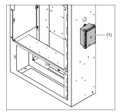
If no LEDs light up when the generator is running, the Cosmos module (1) has not been installed correctly. Consult the Cosmos manual for a description of LED indications.
