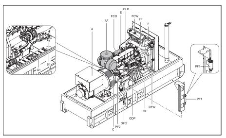
Alternator Α AF Air filter C Coupling DFO Drain flexible engine oil DFW Drain flexible cooling water Е Engine F Fan Filler cap engine oil FCO FCW Filler cap cooling water Fuel filter FF G1 Battery ODP Oil drain pump OF Oil filter OLD Engine oil level dipstick Pre-fuel filter 1 PF1 PF2 Pre-fuel filter 2 S1 Battery switch
