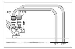
EFT EFR External fuel tank connection
