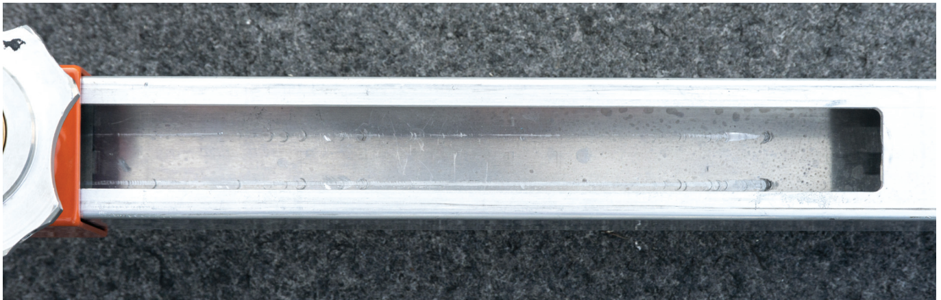
Figure 7, Overload Visual Indicator Marks
