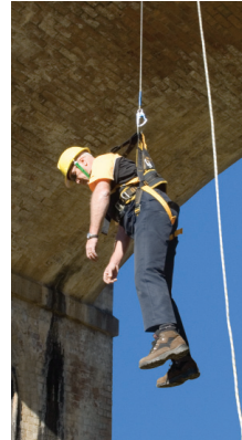
6 Fallen worker descending automatically.
