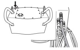
When the power cable and water hoses and hose assembly are connected, the machine can be started.
