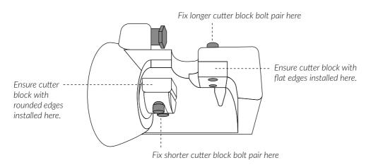
Check cutter block bolts for tightness before each use. Use protective gloves when handling cutter blocks as edges are very sharp.
