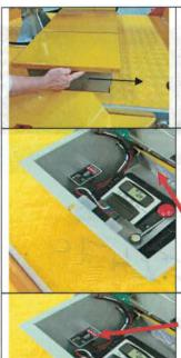
To open the VMS Control box lid, slide the hidden tab to the right as shown.
