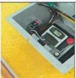
A handle is supplied in the VMS Control box. This is used on the Jack Stands
