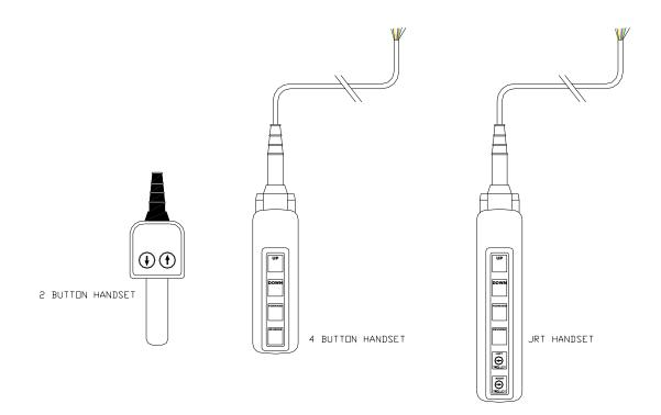
Up and Down (ALL MODELS) To activate the lift or lowering of the boom, press the button on the handset. Select the button
