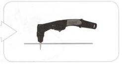
Hold the torch vertically and watch the arc as it cuts along the line.
