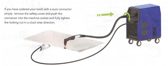
Attach the work clamp securely to the workpiece. Remove rust, paint or other coatings to ensure good electical contact. Attach the work clamp as close as possible to the area being cut to reduce exposure to electromagnetic fields (EMF).
