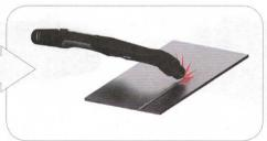
Maintain an approximate 45° angle to the workpiece. Feed into the gouge.
