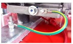
the nuts securely. The other end of the wire should be bolted securely onto an appropriate ground source.
